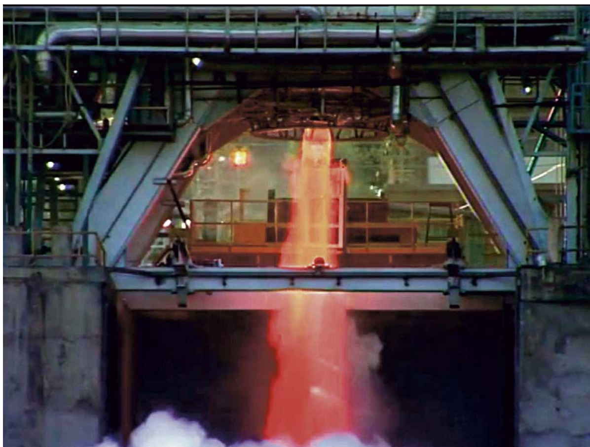
THE SUCCESSFUL TEST FIRING of the cryogenic stage, C-25, for its full flight duration of 640 seconds, at the ISRO Propulsion Complex at Mahendragiri in Tirunelveli district, Tamil Nadu.
